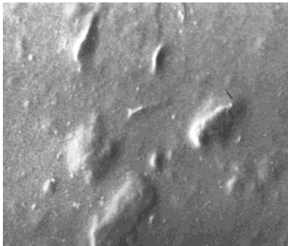
Figure 3 Electron micrographs of the surface of a PDMS(625,000)–PVC blend after treatment with hexane to remove surface PDMS.
